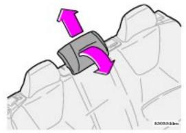
Adjusting center head restraint height-XC70 with optional 3-section rear seat
